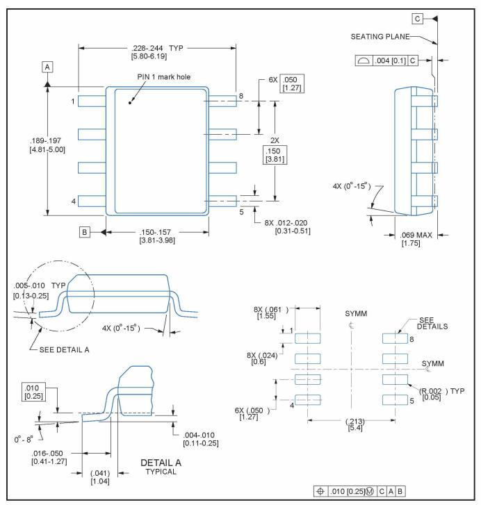
NOTES: Linear dimensions are in inches [millimeters]. This dimension does not include mold flash, protrusions, or gate burrs. Mold flash, protrusions, or gate burrs shall not exceed .006 [0.15] per side.
