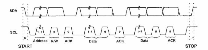
Depending on the status of bit  $R/\overline{W}$ , there are possible two types of transfer:
